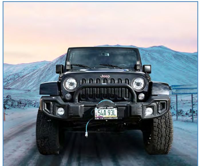
The picture above shows the first Arctic Leash tested for two years for this application. This unit has been submerged, subjected to Arctic temperatures, and 120°F temps. This Arctic Leash shows little to no wear and secure as first installed.
