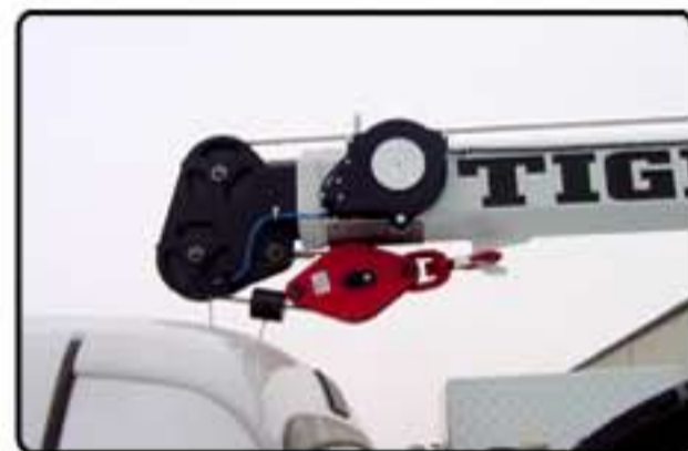
ALLEVIATING EQUIPMENT SHUTDOWNS AS A RESULT OF COLD TEMPERATURES WAS TIGER CRANES CONCERN, THE ARCTIC LEASH SOLVED AN ANTI-2 BLOCK PROBLEM
