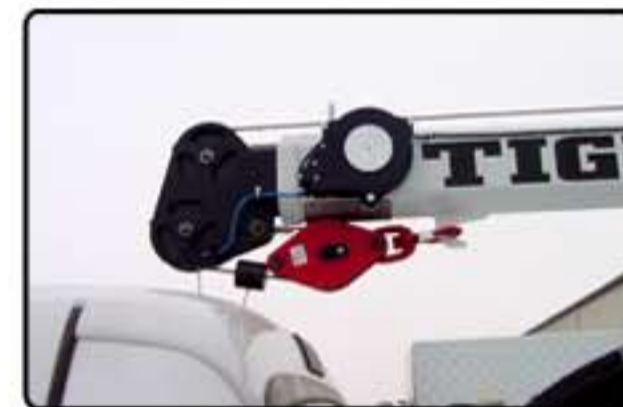
ALLEVIATING EQUIPMENT SHUTDOWNS AS A RESULT OF COLD TEMPERATURES WAS TIGER CRANES CONCERN, THE ARCTIC LEASH SOLVED AN ANTI-2 BLOCK PROBLEM
